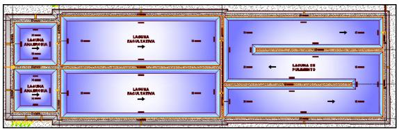
Figure 2. Wastewater Treatment Plant Configuration
