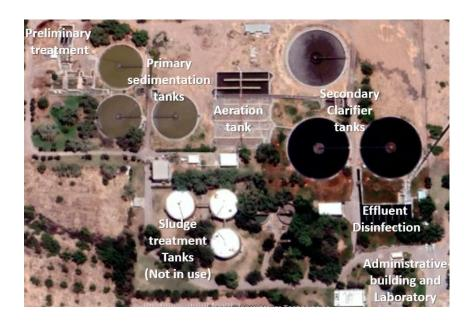
Figure 4 SOUTH WWTP PROCESS
