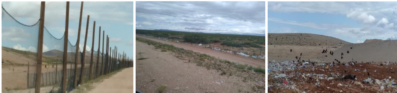
Figure 2.11. Potential problems that may affect water quality: L-R Wind barrier is not effective in preventing waste from escaping the landfill especially after a storm. Waste is getting into the natural environment and can be transported to water bodies. Birds feeding on recently spread waste pile can transfer contaminants to water bodies.
