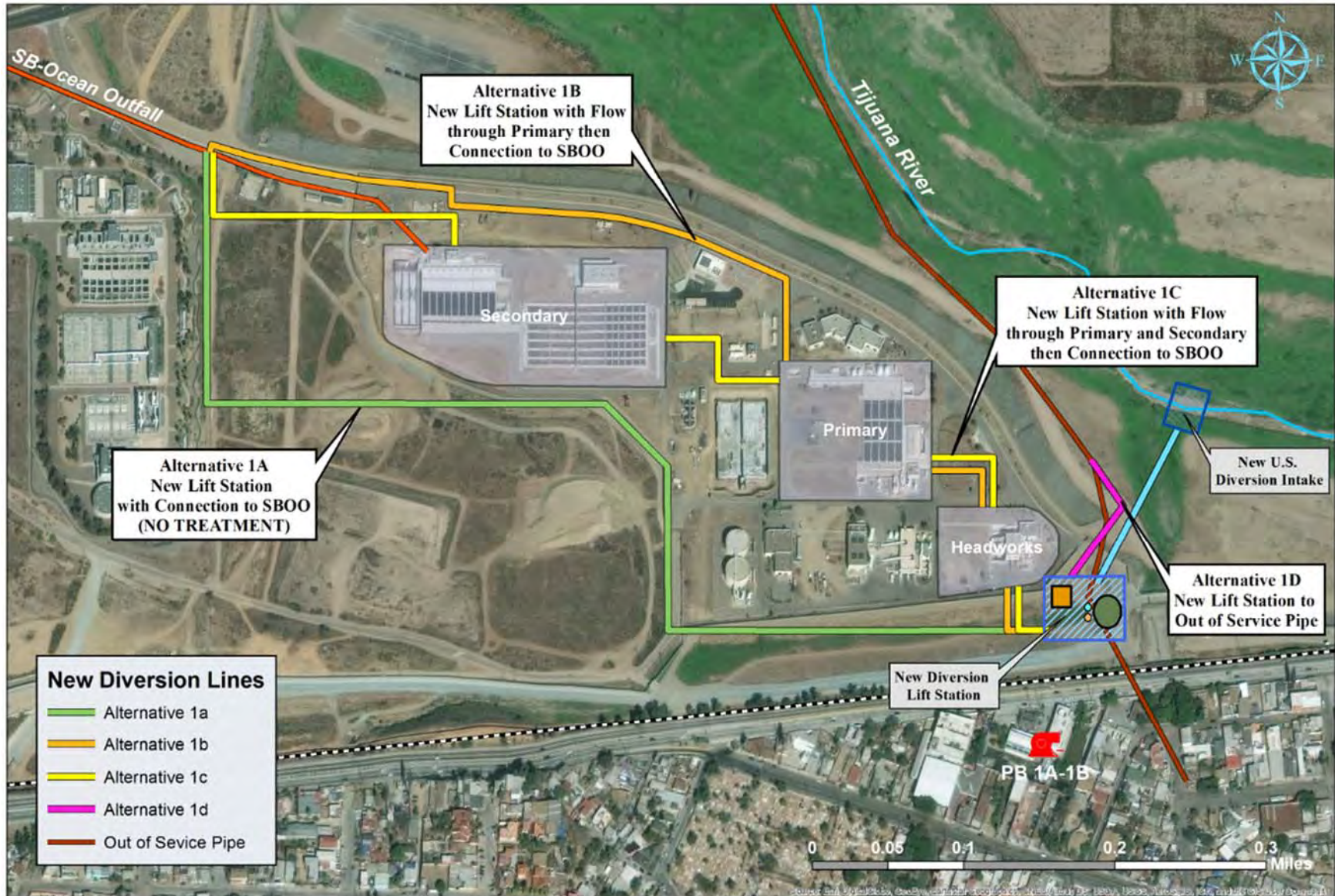
Figure 12. Proposed Lift Station with connections at several locations (Alternatives 1a to 1d)
