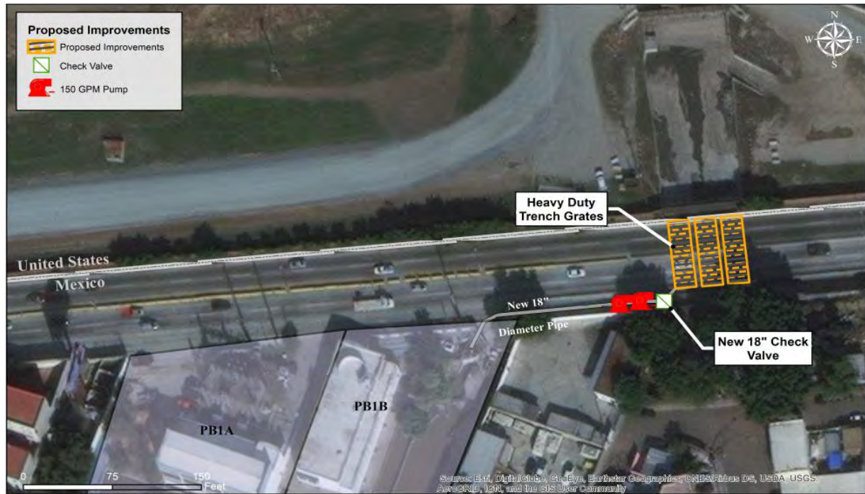
Figure 4-5. Plan view of Stewarts Drain Mexican Based with new grate structure discharging to PB1B.
