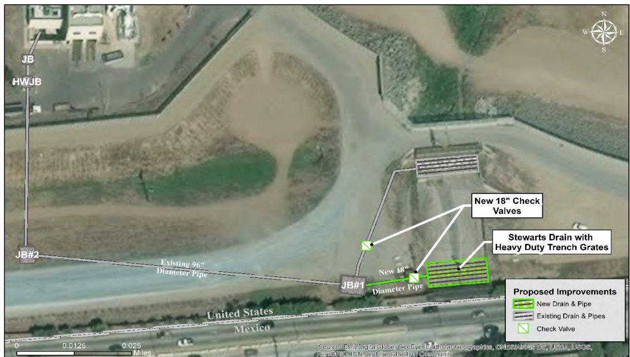
Figure 4-4. Plan view of U.S. based solution at Stewarts Drain with new grate structure discharging to SBIWTP.
