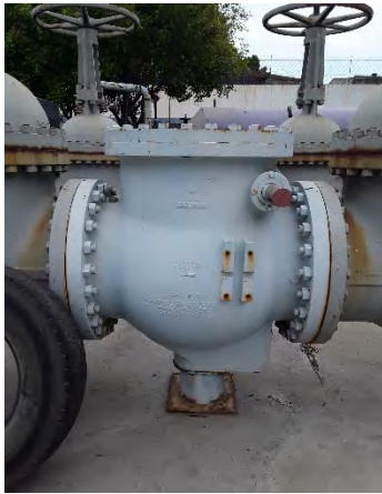
Photograph 15: 24 in check valve for surge control system
