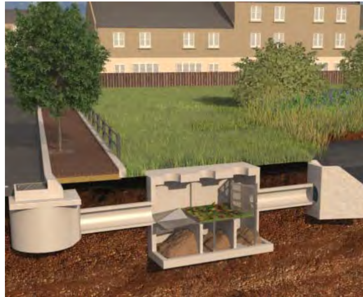
Baffle box with sediment and trash deposition
