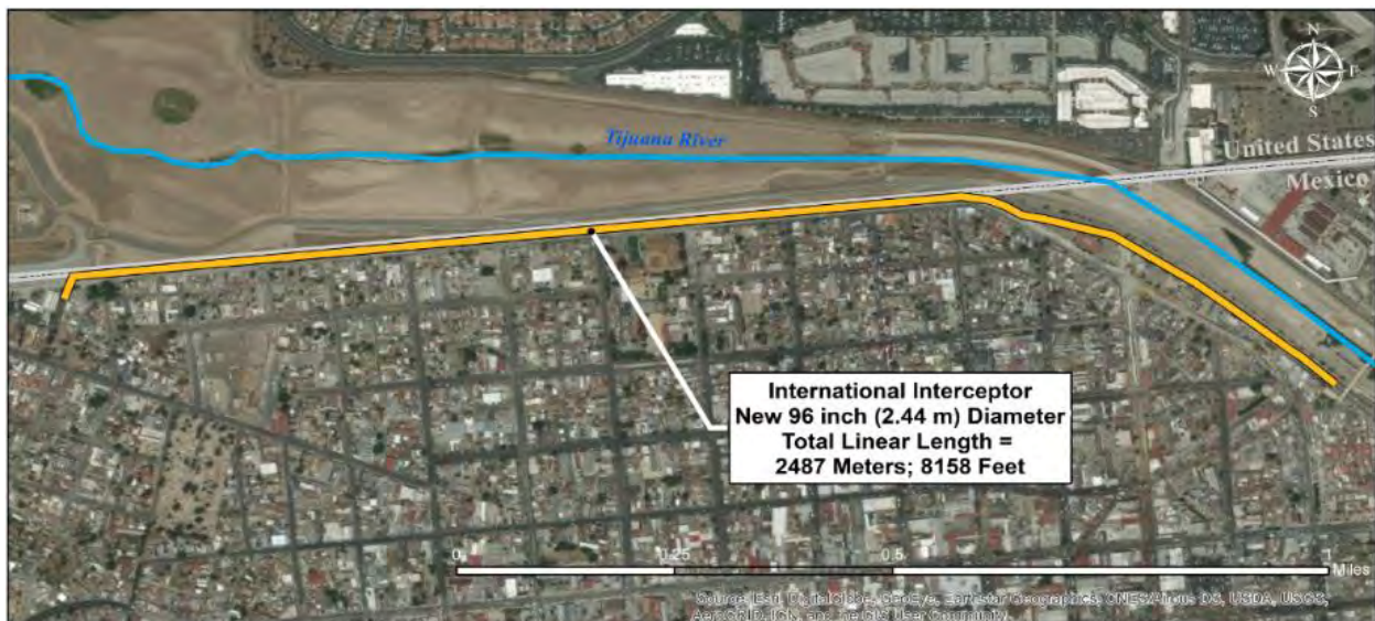
Figure 4-3. Plan view of the International Interceptor location and length.
