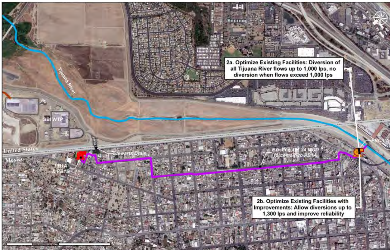
Figure 3-14. Optimization of existing facilities (Alternatives 2a-2b)
