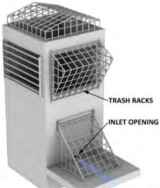
Concrete riser with racks
