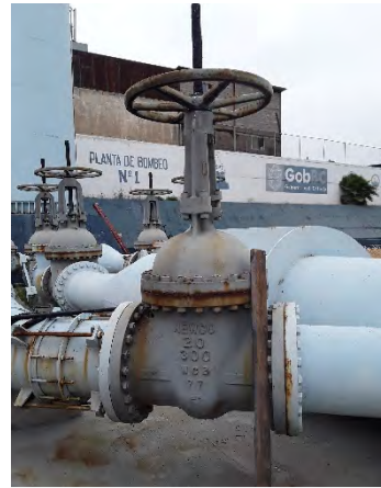
Photograph 16: 24 in gate valves for surge control system
