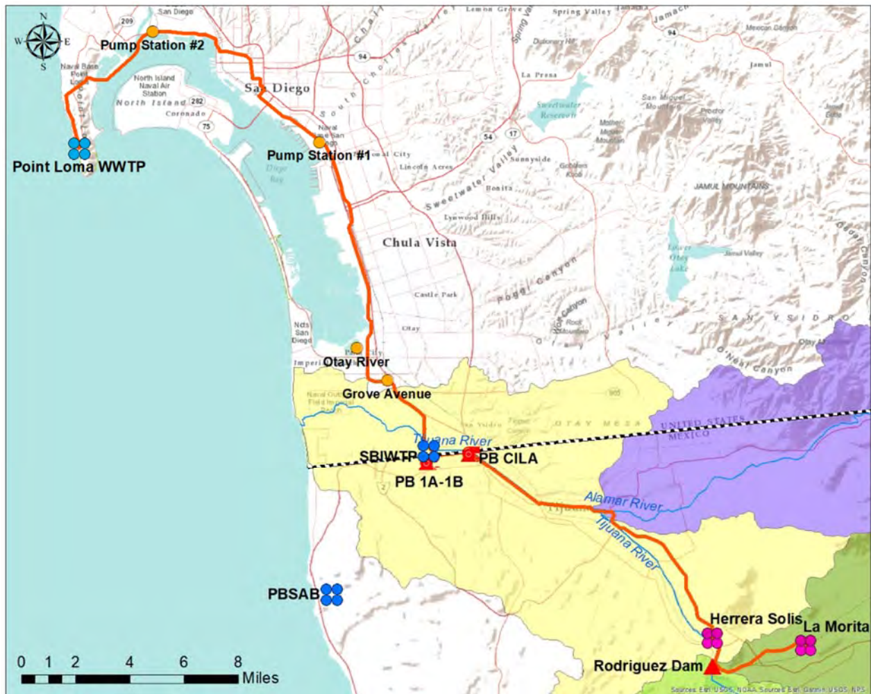
Figure 15. Reclaimed Water pipeline connecting to Point Loma WWTP force main (Alternative 2b)
