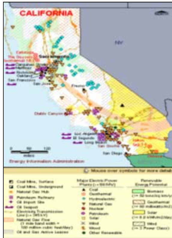
Figure 3. Location of electrical plants and potential renewable energy sites in the state of California.
