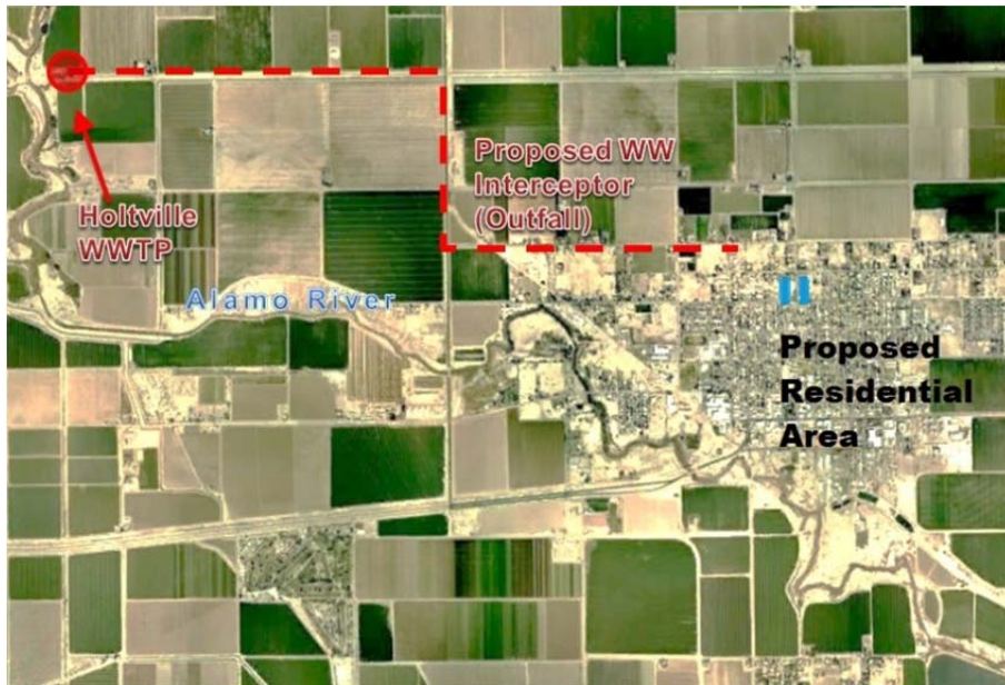
Figure 2 WASTEWATER OUTFALL and RESIDENTIAL COLLECTION SYSTEM PROJECTS
