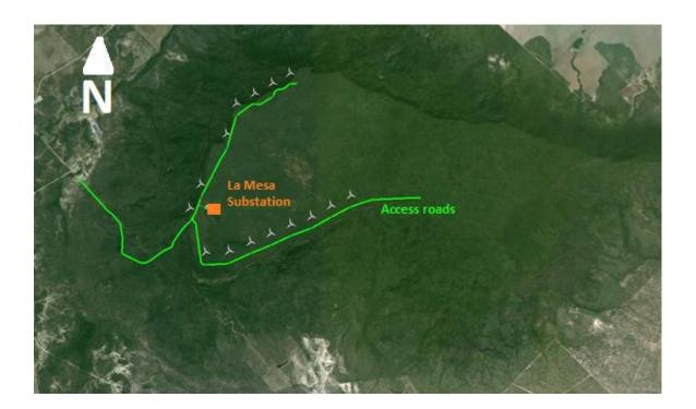
The Project components include the installation of wind turbines, one substation and a transmission line. The energy generated by each wind turbine will be conveyed to the substation through 34.5 kV underground lines. The Project will be interconnected to CFE's Nuevo Santander substation through a 115 kV overhead transmission line extending 25.3 kilometers (15.7 miles).
