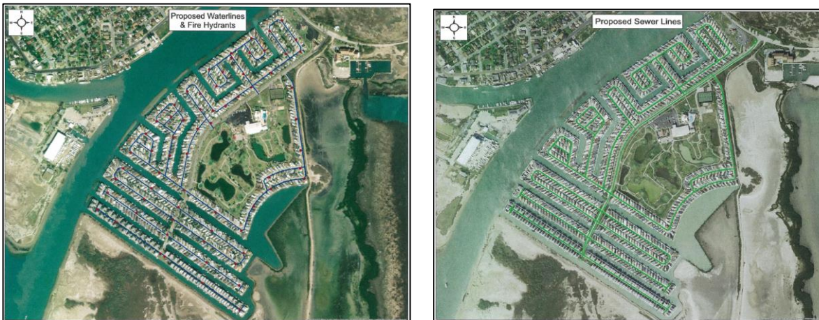
Figure 3 PROPOSED WATER AND WASTEWATER INFRASTRUCTURE LAYOUT
